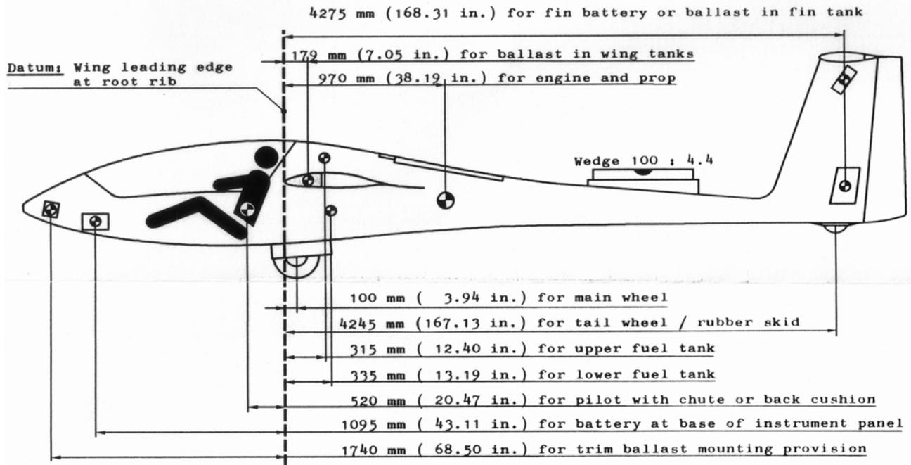
10.3 Worked example 1: In the aircraft above, calculate the change of in-flight CG due to a reduction in pilot weight of 10.0 kg, which is to be compensated for by adding 3.0 kg at the nose trim ballast location.
