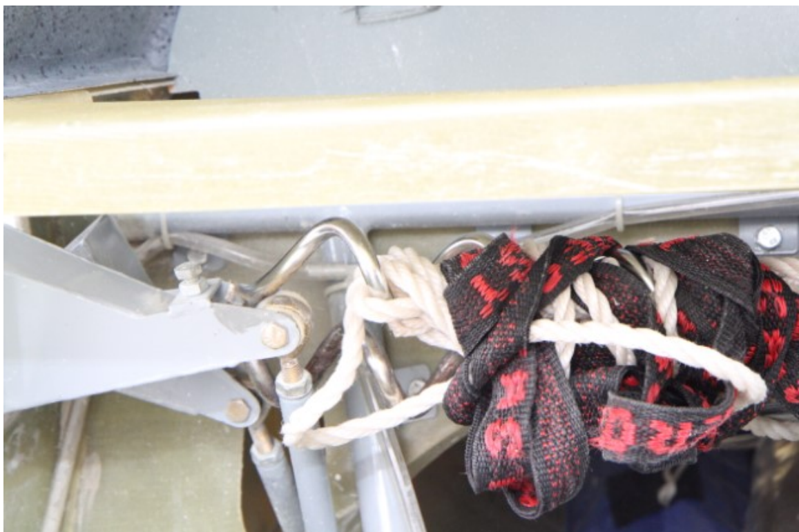
Picketing equipment jammed in the centre fuselage flight control system.
