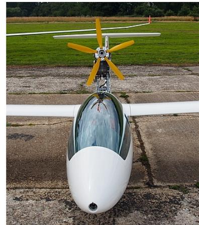
*Typical Schempp-Hirth glider with sustainer motor extended*
