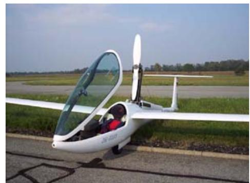
In order to retract this assembly, the propeller must be folded, OR stopped and aligned vertically, to allow complete retraction into the fuselage. The alignment may be accomplished electrically, or by using windmilling and a brake to achieve the correct position. Whatever system is used, the Flight manual procedures must be diligently followed. It is highly recommended that pilots practice these procedures on the ground before attempting them while flying.
