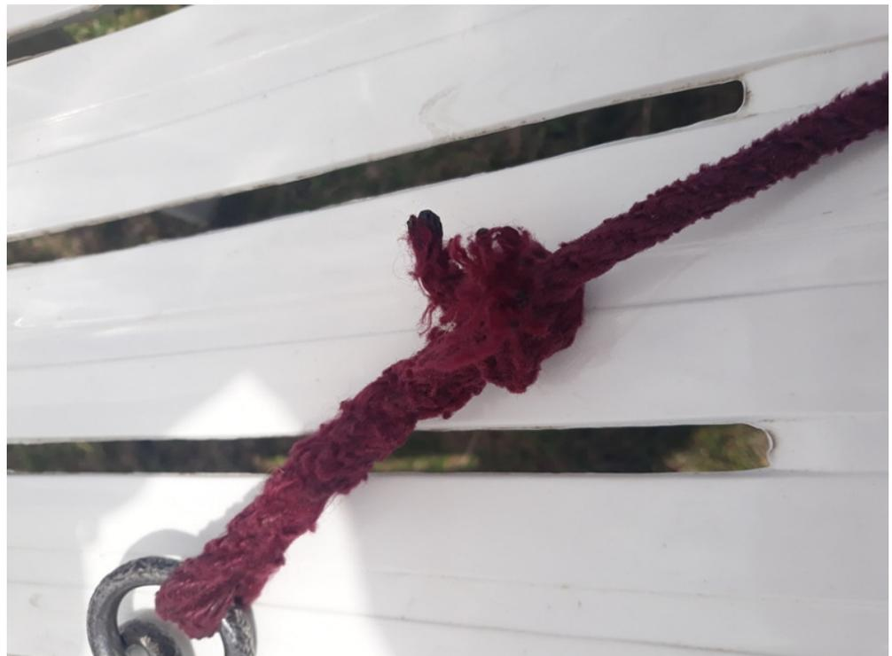
**THERE IS A KNOT IN HERE.....AT THE END OF THE SPLICE.....AND WE TOWED WITH THE ROPE LIKE THIS.** Be careful, have a good look and feel. This was hard to see and impossible to get out. Neville cut the section out and respliced.
