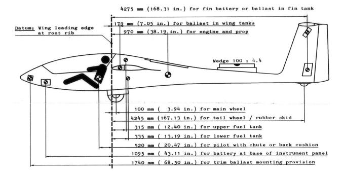
10.3 Worked example 1: In the aircraft above, calculate the change of in-flight CG due to a reduction in pilot weight of 10.0 kg, which is to be compensated for by adding 3.0 kg at the nose trim ballast location.
