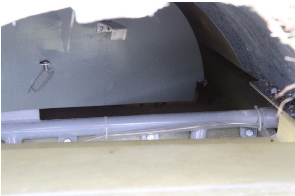
Stowage tray bulkhead to main fuselage detail.
