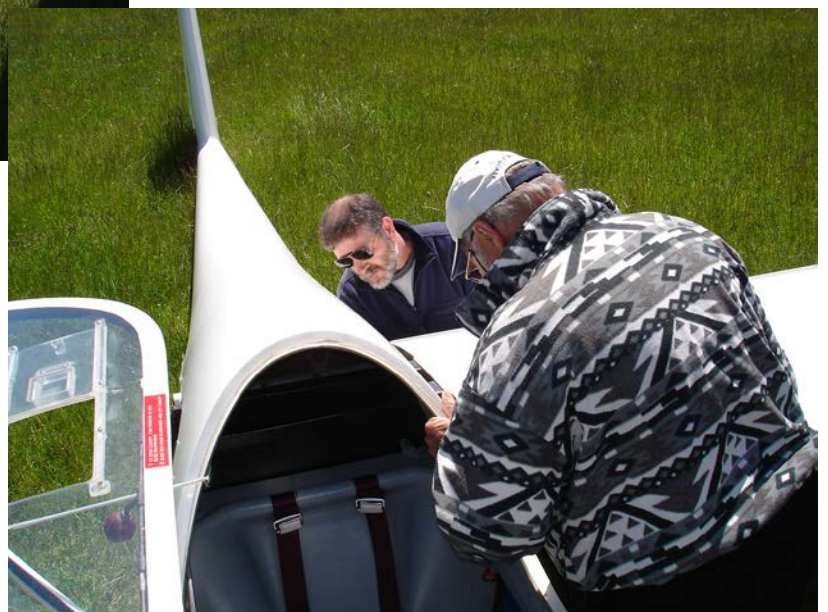
Wing roots are heavy... make sure there are ample strong people to hold them as the wing is removed from the fuselage and that the fuselage is well supported, in this instance, it is in a fuselage cradle
