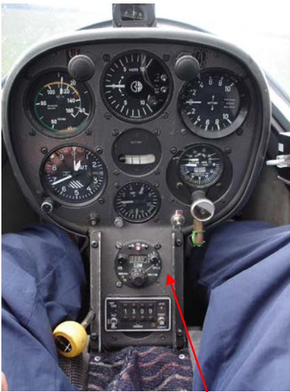
A typical radio installation
