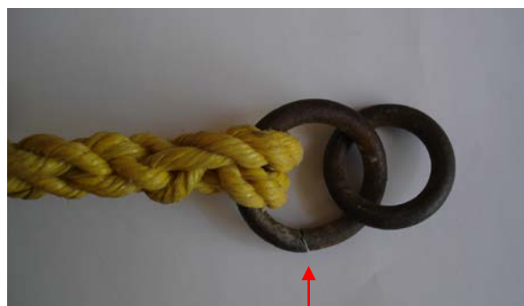
Spot the crack in the big ring
