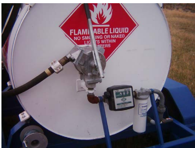
A typical “wobble pump” hand pump system
