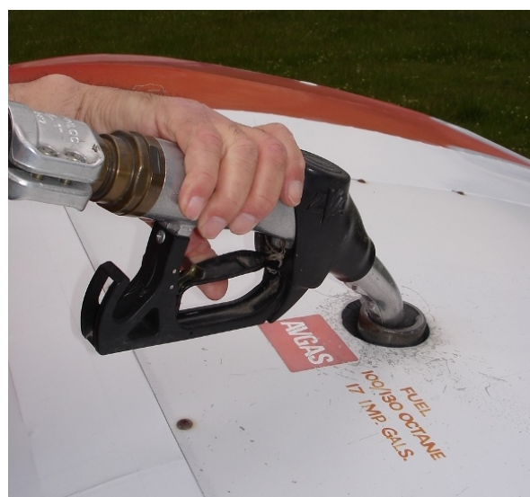
Hold the fuelling nozzle securely to prevent spillage
