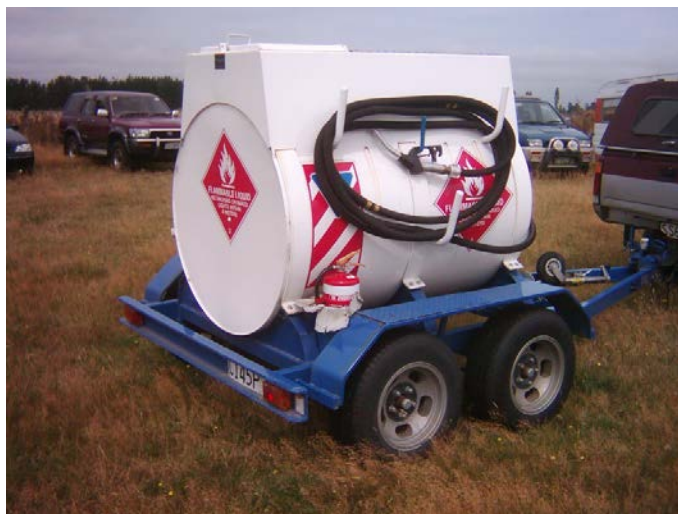
A trailer mounted fuel supply
