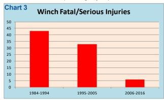
Fewer fatal or serious injuries from winch launches has been driven by fewer injuries from an accelerated stall during rotation, from a stalled landing after launch failure below 100ft, and from a spin after launch failure in mid launch. There were 3 such stall/spin injuries in the most recent 11 years compared with a previous 11-year average of 31 such injuries.
