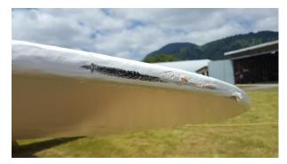
Hangar Rash is caused by - being too impatient & rushing, not having enough people to assist and not correctly setting up the hangar doors before removing the aircraft.
