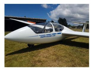
It was decided to start doing the 3000 hour check at the same time which is nearly complete. Basically all that is left to do is to renew the rudder control cables which will be organised at a later date. Once completed, GTG will be good to go for another 3000 hours.
