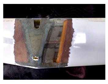
As you can see below there are a lot of layers of fiberglass near the center and it tapers out into the foam. Here we have removed a rectangular section of the foam.
