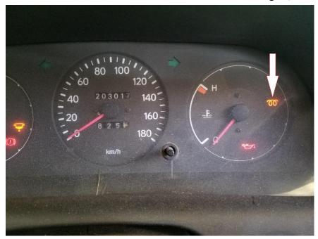
glow plug light has gone **OUT** before you crank the engine. Excessive cranking has been one of the major factors as to why the starter motor failed in the first place.
