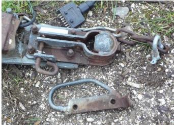
For I do not know how many kilometres, the trailer coupling had been floating freely on the tow ball! Fortunately a replacement bolt was obtained from the petrol station workshop to secure the lever for the remainder of the trip.
