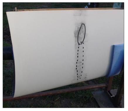
Several bits inside the wing were also loose and rattling about. Closer inspection showed that the wing skin along the row of cracks had been crushed internally and the structural integrity across the full width of the tail plane was compromised.
