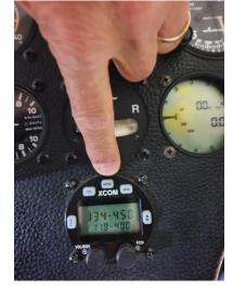
The display will then show battery voltage. Press the Push to Talk button and you will get the true voltage reading. If the battery indicates less than 12V, change it out with a charged battery.
