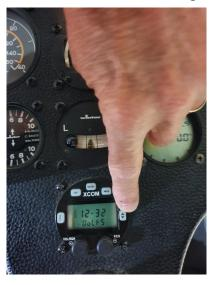
To switch back to the radio frequencies, press the toggle switch on the right.
