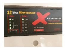
3. CHECK BATTERY VOLTAGE and **RECORD VOLTAGE LEVEL** in THE BATTERY'S LOG
