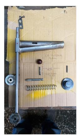
that was around the wrong way allowing the ball to rub on the pedal. It is shown around the correct way.
