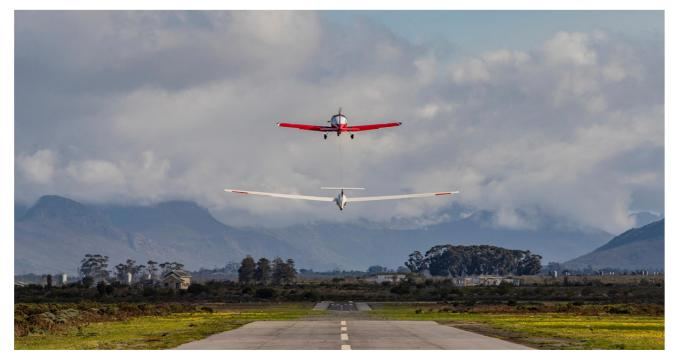
Much like a see-saw, if the glider gets high the weight being exerted by the glider to the towplane is raising his tail because we are essentially lifting it up. And if that tail is getting high, his nose is getting forced down.
