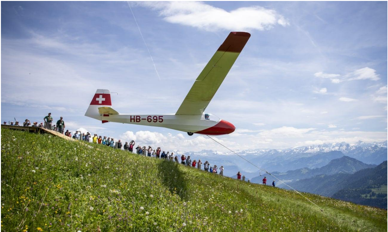
Schleicher K-8B launches for a flight of many hours, aided only by a small bungee. Thun, Switzerland
