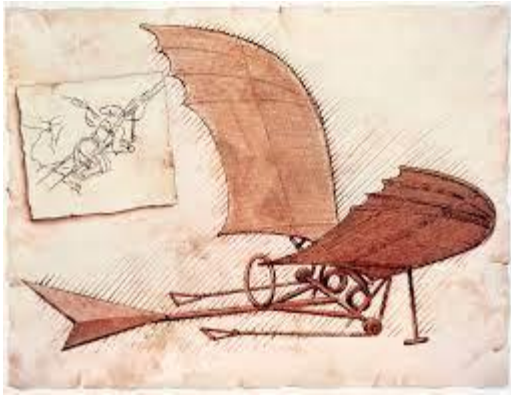
Leonardo's glider drawing. Note the avian wingshape and lack of a vertical fin
