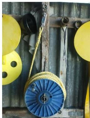
**DO** - Hang the tow ropes up at the end of the day so that the weak link is secured to the nail. This ensures that the link is visible and can be checked for any elongation.
