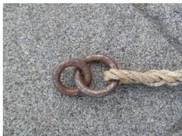
**DO NOT** tow the gliders with a rope that does not have the correct ring set up such as the rings in this photo.
