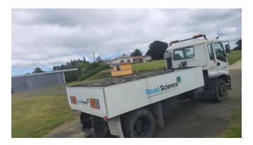
Every 10m the truck stops to compress the pavement, whilst one end of a beam sits between two rear wheels.
