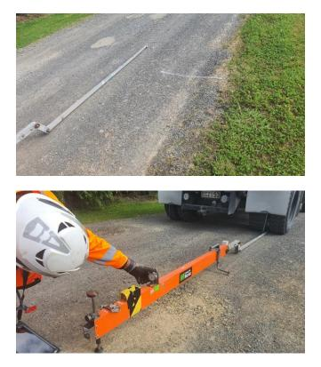
The truck then drives forward and a dial gauge at the other end of the beam measures the amount the pavement returns back up. This gives the pavement deflection.
