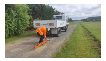
Pavement deflection, measured every 10m along the driveway length, provides a picture of how even the substrate is and identifies where the soft patches are located. The subgrade is then treated accordingly, to even out pavement deflection to within a specified tolerance.
