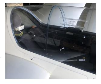
It appears that the glider had dived below the falling winch cable, then the nose of the glider snagged the cable as it slowed down. The dyneema cable ended up lying across the rear canopy and under each wing, and was dragged across the canopy by the tension from the opened parachute. This heated and deformed the plastic.
