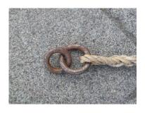
**DO NOT** tow the gliders with a rope that does not have the correct ring set up such as the rings in this photo.
