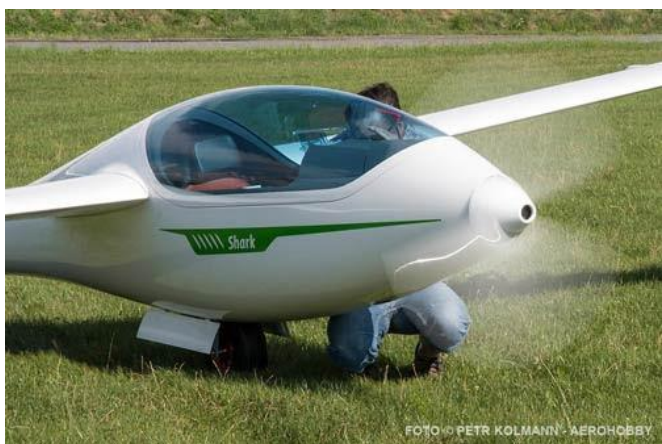
Photo by Petr Kolmann of a HpH 304 ES Front Engine Sustainer (FES)
