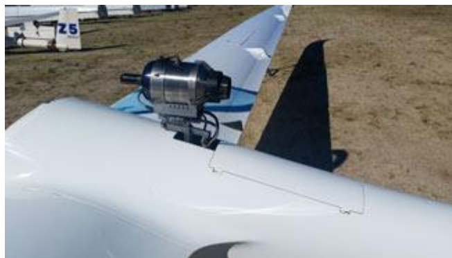
Photo by Sean Franke of a HpH 304 SJ Jet Sustainer Engine
