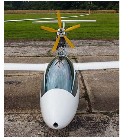
Typical Schempp-Hirth glider with sustainer motor extended
